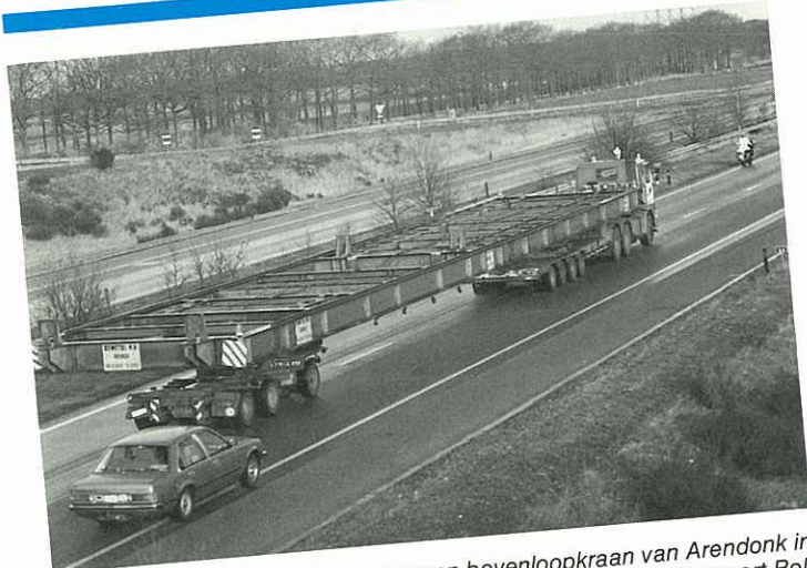
In January 1984 this overhead crane was transported by Mammoet Transport Belgium from Arendonk, Belgium to Waspik, Holland. It weighed 45 tonnes, was 41 metres long and 5.4 metres wide.
